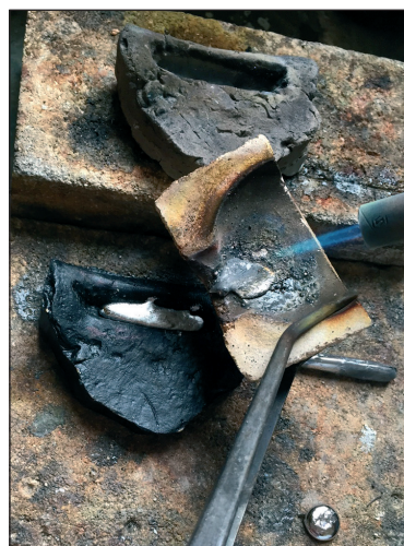
■ Obr. 10 Odlievanie olova do formy.
