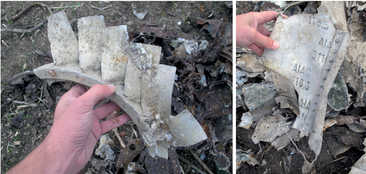
Fig. 36–37 Other interesting finds, which always safely identify the Me 262, included engine blades or a cover plate with the manufacturer's marking (AIAG, Aluminium Industrie, AG Zürich) on the inside.
