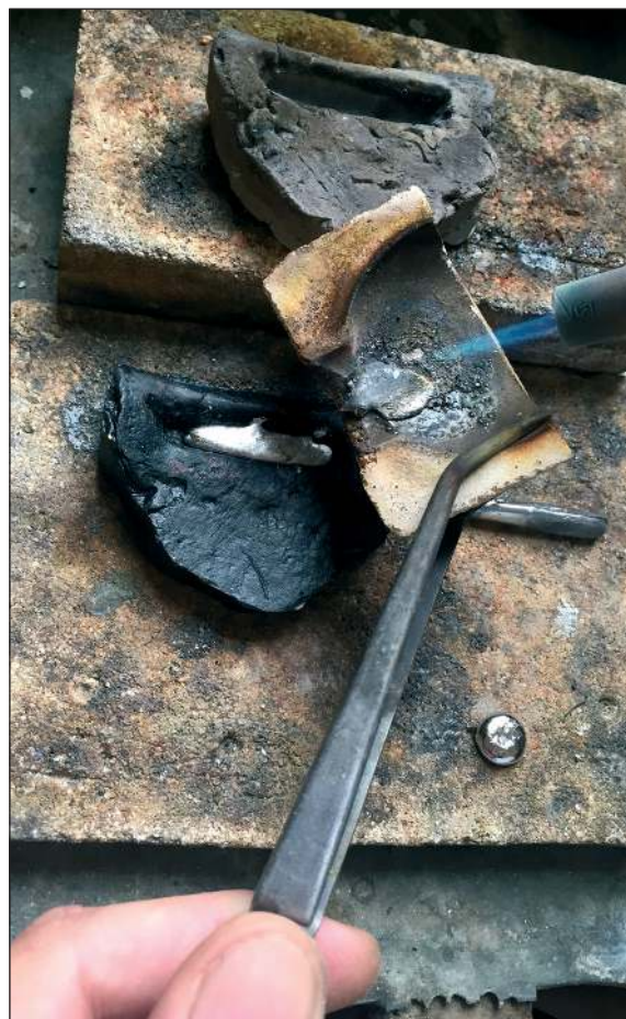
■ Obr. 10 Odlievanie olova do formy.
